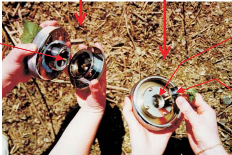
SKPM 1445 Specimen holding adapter. Choice of 3 sizes. Change using the 4 screws
