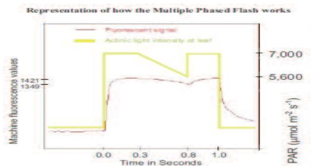
A multi-phase saturation pulse technique (Loriaux 2013\*) to determine  $F_M'$  is provided to ensure accurate measurements of Y(II) and ETR on leaves with a high light level history.
