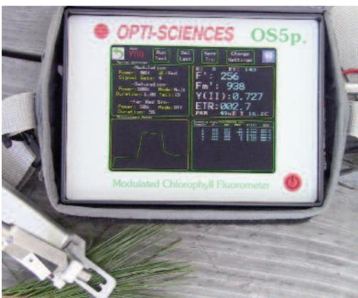
Data can either be stored in the large 1Gb internal memory, capable of storing thousands of test data sets and traces, or on removable SD memory cards. Data may also be downloaded via a USB port.
