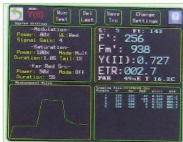
**Quantum Photosynthetic Yield Y(II):** Also referred to as light adapted quantum yield of PSII. The most widely used light adapted test, sensitive for most types of plant stress. Y(II) reduces under stress. The OS5p+ features multflash  $F_M'$  correction ensuring accurate measurements even for leaves with a high actinic light history.
